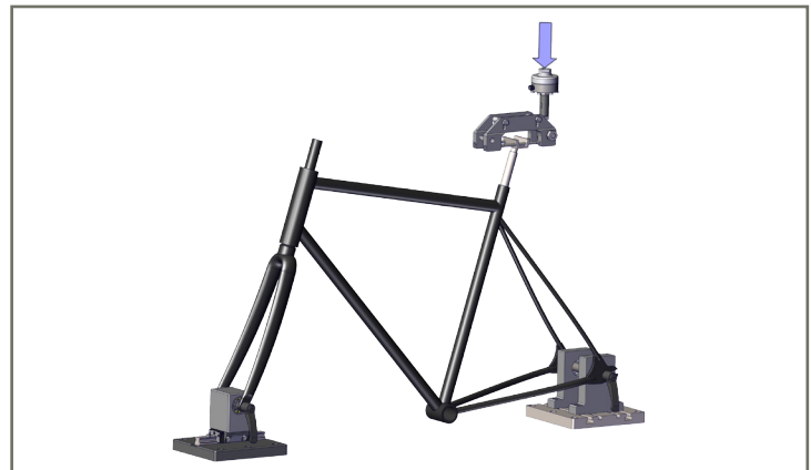
Frame: seat post vertical stiffness test
